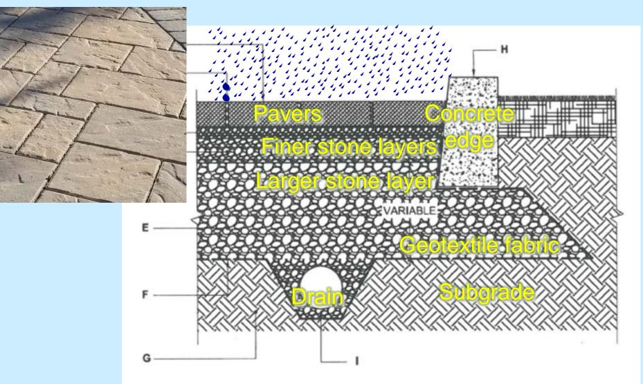
Example of permeable pavement design by Techo-Bloc
