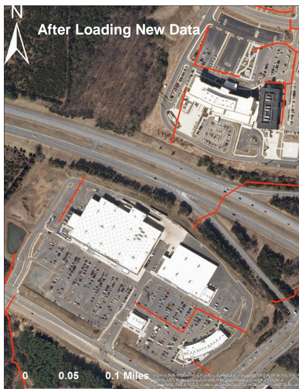
Figure 8. Depicts post-2009 development along Highway 15 and I-66 in Haymarket, VA. The image on the left shows the location in 2009, while the image on the right shows the area in 2015 after loading the new data into the Amec Single Network. Newly added segments still require editing to create a hydrologic connection. Editing procedures for creating this hydrologic connection are described below.
