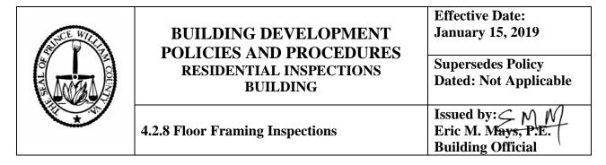
Residential Floor Framing Systems that are less than forty-two (42) inches above the finished grade require an approved Residential (114R) Building Concealment Inspection prior to the installation of the floor sheathing or decking materials. The measurement is taken from the bottom of the lowest floor-framing member to finished grade.
