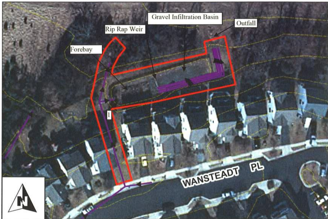
Existing Condition: Facility in need of maintenance and possible retrofit
