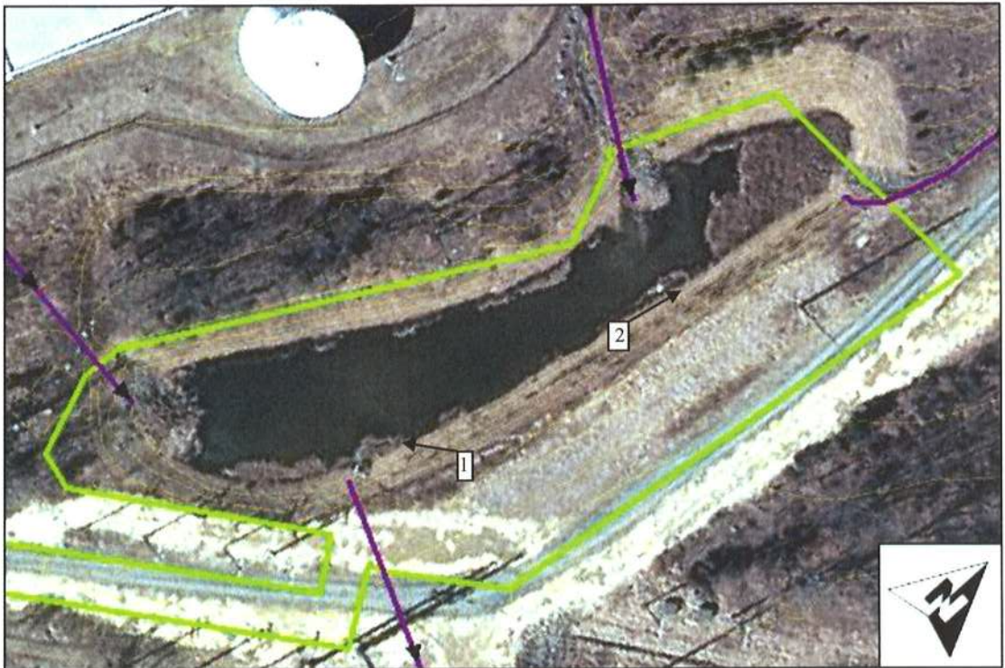
Existing Conditions: Dry basin BMP with permanent pool and wetlands
