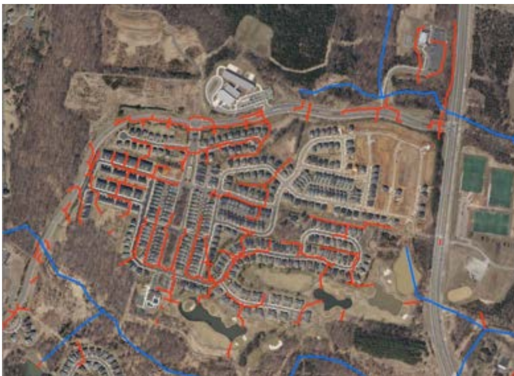
Figure 9. This view shows what the user would see after loading in a new set of stormwater infrastructure into the geodatabase. MS4 outfalls and hydrologic connections still need to be added by the user. Note the stormwater infrastructure is a discontinuous network within itself, but also lacks continuity with the NHD Flowlines.
