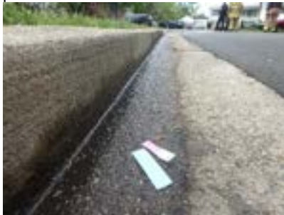
Water paper and oil finder paper testing on spill in front of 4707 Kenny Court
