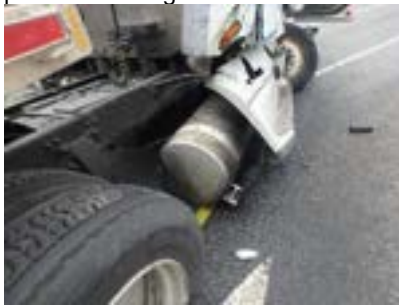
photos:Diesel fuel leak
