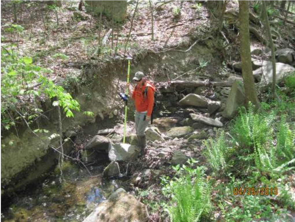
43. Looking upstream at a typical section of Stream Reach 12. This portion shows significant incision along the banks.
