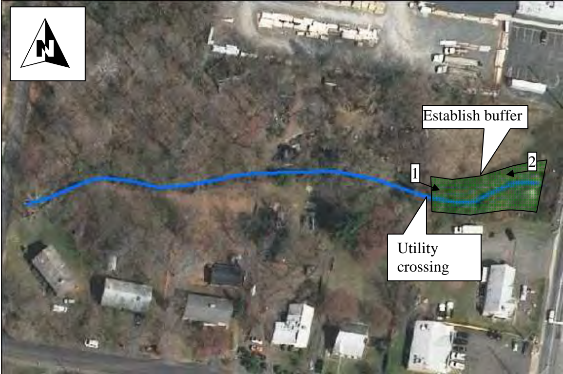
Conceptual Plan: Stabilize stream at utility crossing and establish buffer
