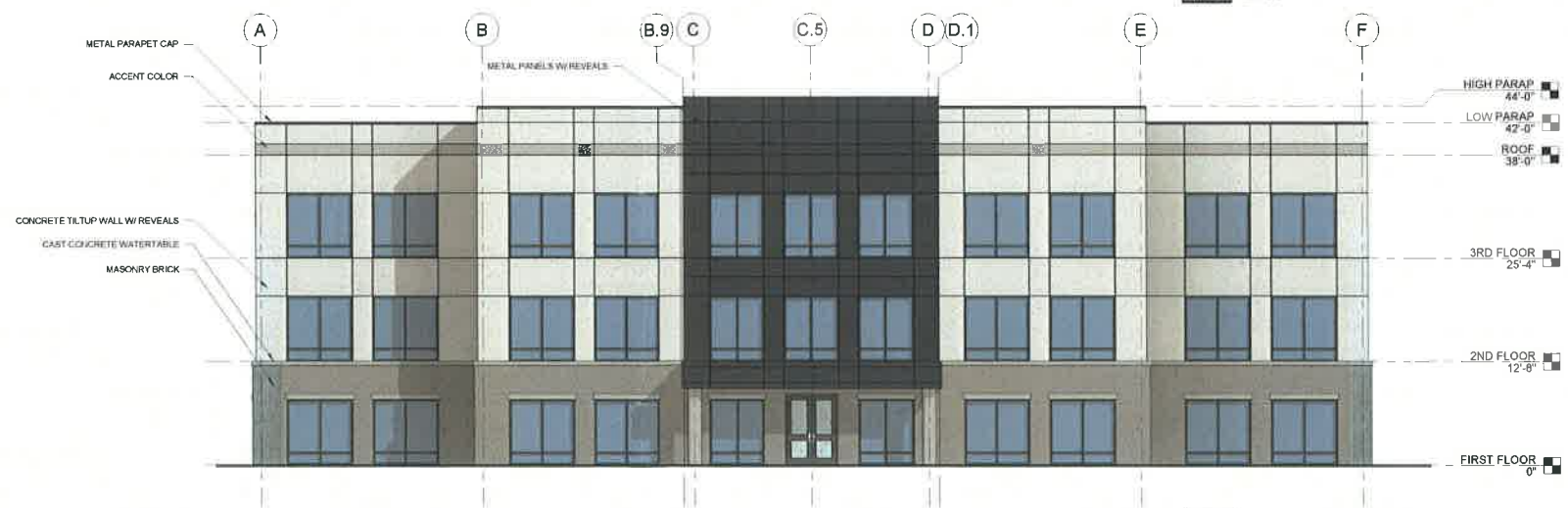
1 OFFICE - FRONT ELEVATION SD1.0 1/8" = 1'-0"
