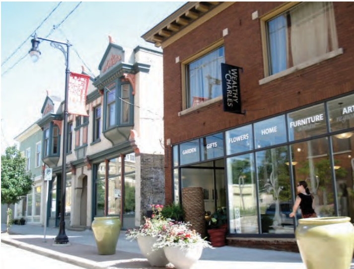
Base should have greater level of transparency than the middle or top.
